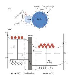
**Figure** 5: (a) Schematic model for the p-type NiO/n-type  $SnO_2$  heterostructure based sensor when exposed to acetone. (b) Proposed band structure for p-type NiO/n-type  $SnO_2$  heterostructure.  $E_c$ : lower level of conduction band;  $E_f$ : Fermi level;  $E_c$ : upper level of valance band.
