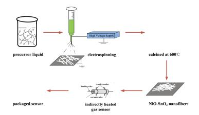
Figure 1: Schematic of the fabrication process of NiO-SnO<sub>2</sub> composite nanofibers based gas sensors.
