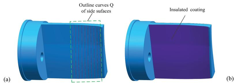
**Figure 5:** Side surface construction (a) and insulated coating (b).
