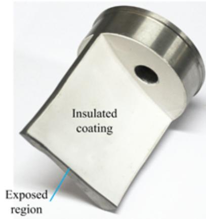
Figure 7: Result of designed cathode.
