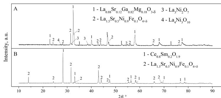
Figure 1: XRPD patterns of  $\text{La}_{1.5}\text{Sr}_{0.5}\text{Ni}_{0.9}\text{Fe}_{0.1}\text{O}_{4+\delta}$ -LSGM (A) and  $\text{La}_{1.5}\text{Sr}_{0.5}\text{Ni}_{0.9}\text{Fe}_{0.1}\text{O}_{4+\delta}$ -SDC (B) mixtures after calcination at 1250°C for 1 hour.
