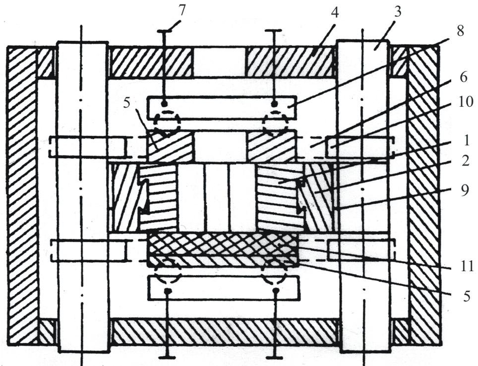
**Figure 1:** Design of the facility for continuous casting and deformation of metal. (1) Sidewalls, (2) support, (3) driving eccentric shafts, (4) frame walls, (5) upper and lower walls, (6) articulating system, (7) clamping facility, (8) flat ball bearing, (9,10) eccentrics, and (11) insertion from a material with low thermal conductivity.
